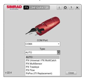
With the PX Configurator program, you can configure and change the parameters of the following catch monitoring sensors:
