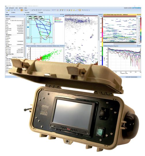
frequencies is ideal for mapping ecosystem components and separating fish from plankton. The 38 kHz is also split-beam for accurate target strength measurements and target tracking.
