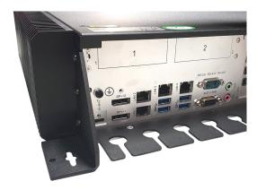
Fasten the two mounting brackets to each side of the rear panel. Mount the cable retaining plate.
